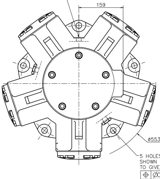
REVERSE PORT CONNECTIONS FOR OPPOSITE DIRECTION OF SHAFT ROTATION
